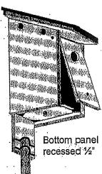
Vent holes and front slot keep interior cool
