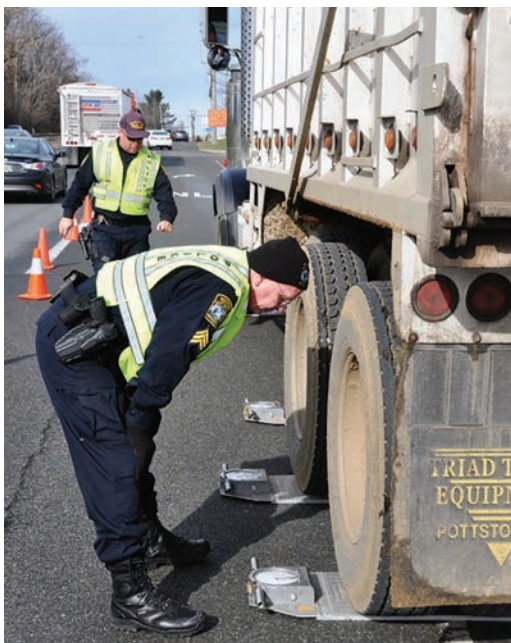
Sergeant Leo Kennedy (forward) and Officer Gary Frey (back) set the individual scale pads under a dump truck.
