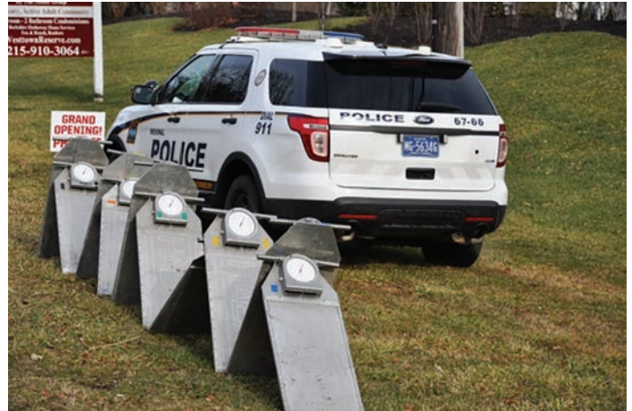
Scale sets are staged in pairs for use during the commercial motor vehicle inspection detail.
