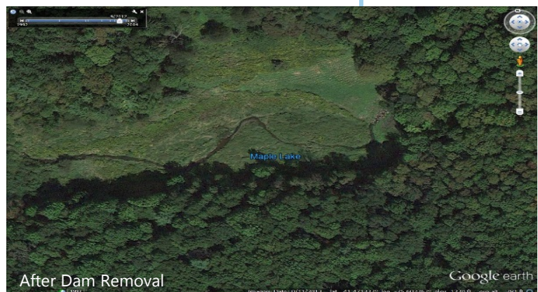
Figure 2-10: Maple Lake Dam Breach. Gannett Fleming determined that breaching Maple Lake Dam, which was no longer used for water supply, was more cost-effective than rehabilitating the high hazard structure.
