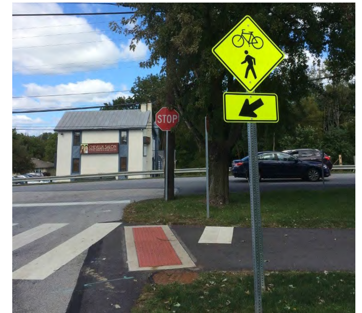
Example of signage and gates for a trail crossing of a roadway or driveway
