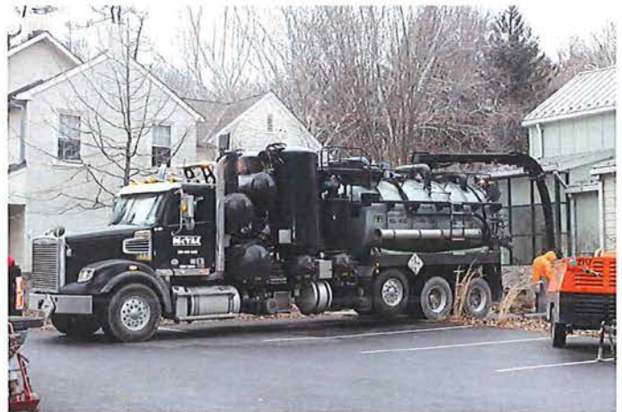
Vacuum trucks can be used to clean out ponds where sediment is more localized in forebays. This can be a less costly option than dredging.
