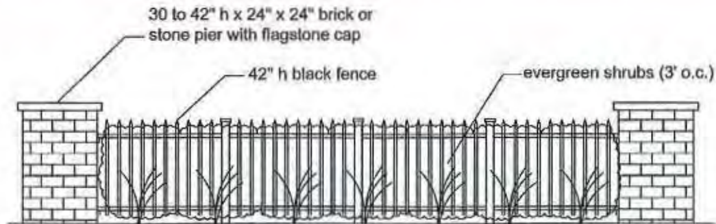
Typical Section of Pier, Fence & Hedge
