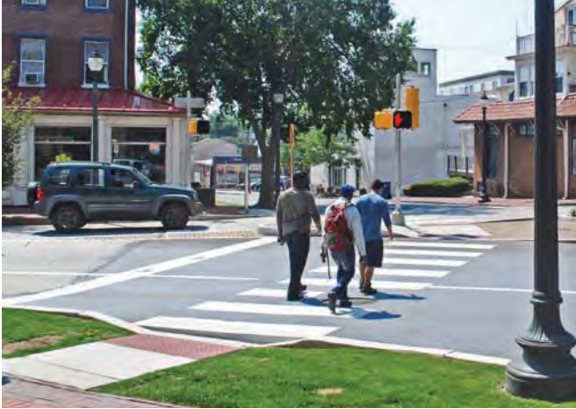
Crosswalk Striping connecting opposing accessible sidewalk ramps
