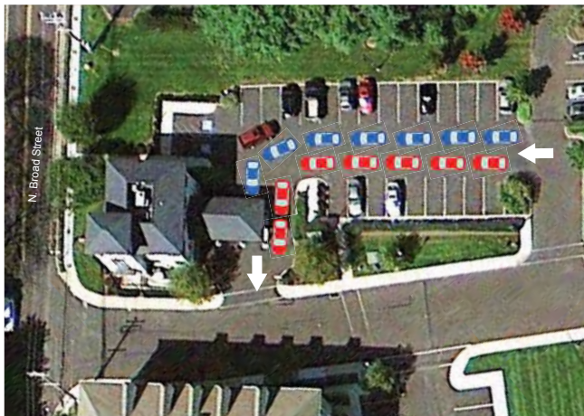
Traffic Stacking at Drive-Thru Facility located in the rear
