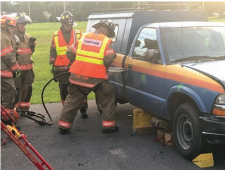
Hydraulic tool is used to force a door open. Note the "cribbing" under the truck that will hold it in place
