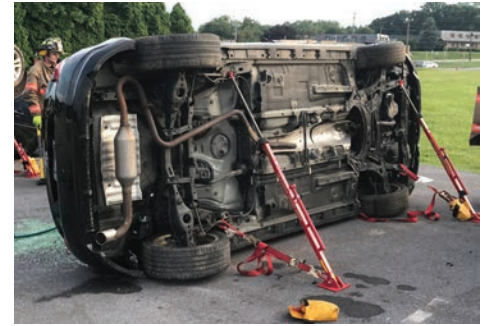
Vehicle that has rolled on its side has been stabilized
