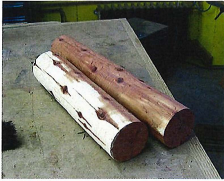
A log sawn in two and turned on a lathe, exposing the pale sapwood and the reddish heartwood
