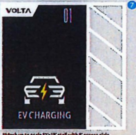
*Mock up to scale 12'x14' stall with 5' access aisle.
