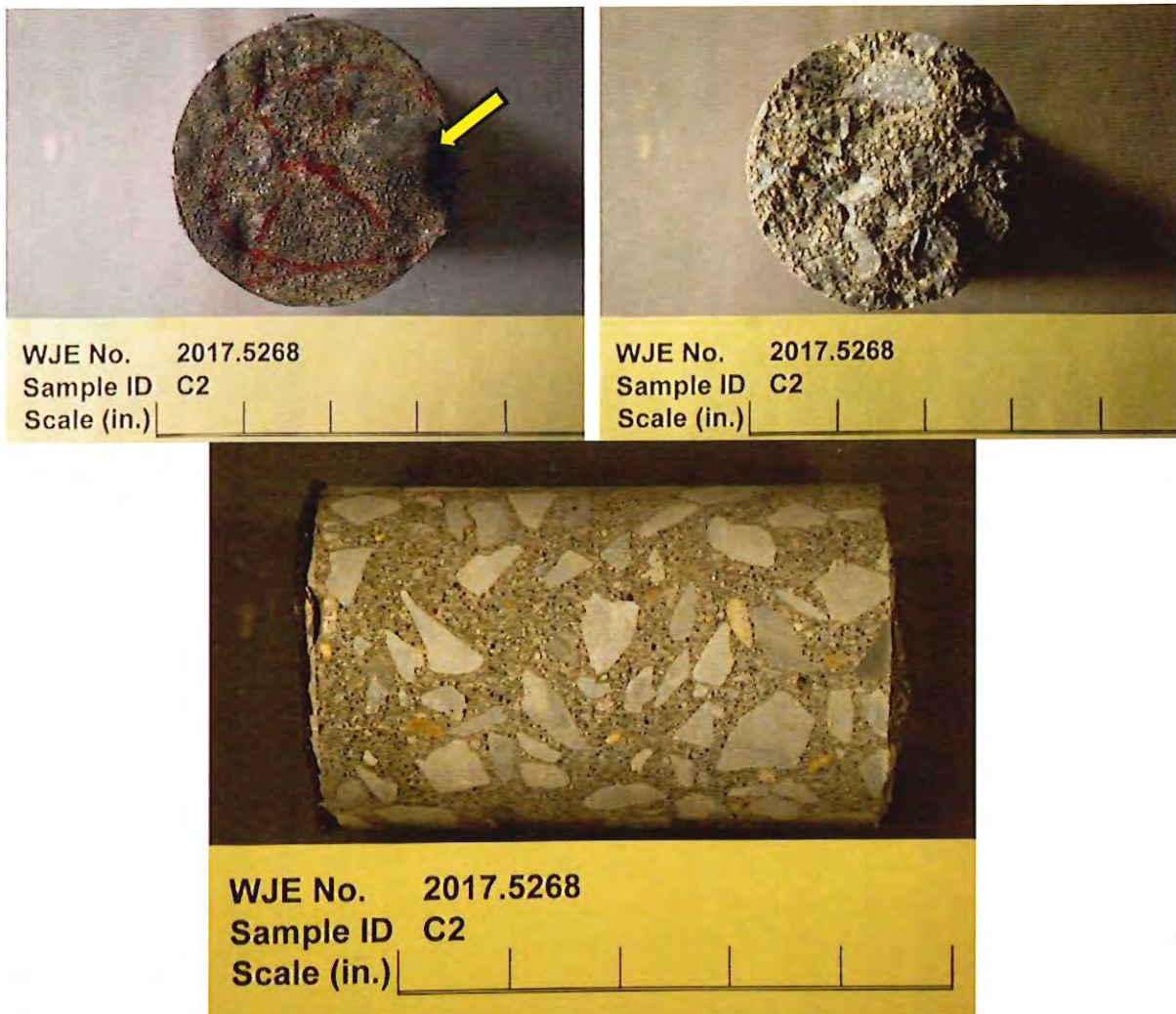
Figure 3. The as-received appearance of the exterior coated surface (top left), the interior fracture surface (top right), and the side of Core C2 is pictured. A blister on the exterior surface of Core C2 is identified with an arrow.
