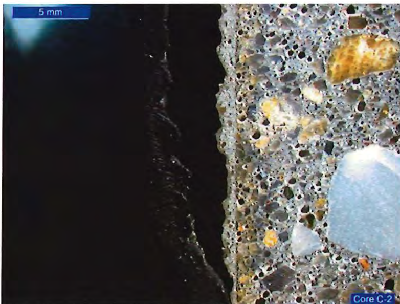
Figure 21. The irregular surface profile of the skim coat is reflected on the inboard surface of the coating at the blister, indicating that the materials had been in contact prior to the blister formation.
