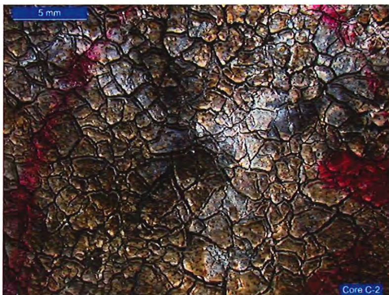
Figure 7. The exterior surface of the coating exhibits an "alligator cracking" pattern, pictured for Core C2.
