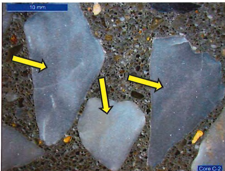
Figure 25. The concrete contains crushed limestone coarse aggregate (arrows) and manufactured siliceous sand fine aggregate.
