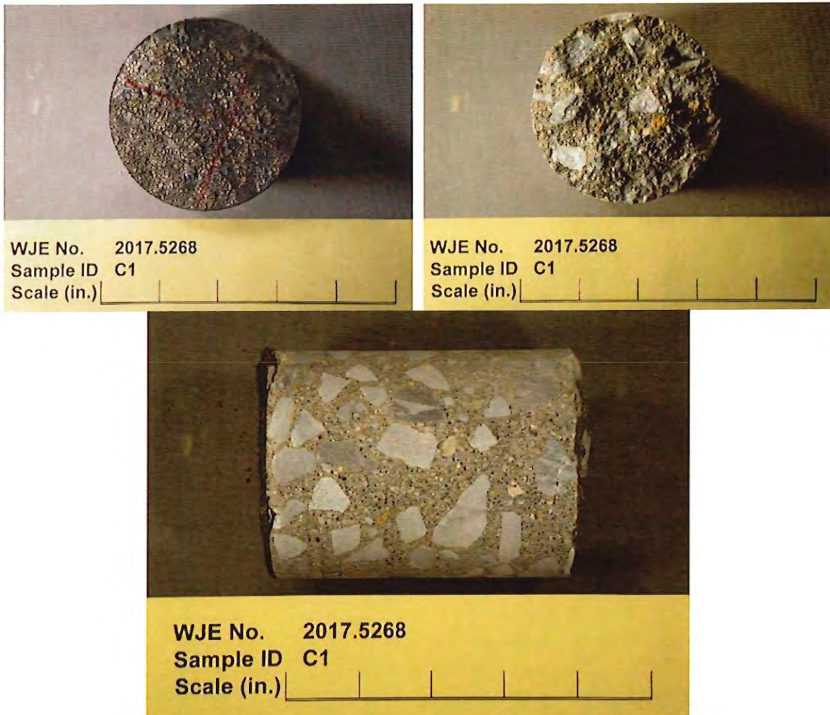
Figure 2. The as-received appearance of the exterior coated surface (top left), the interior fracture surface (top right), and the side of Core C1 is pictured.
